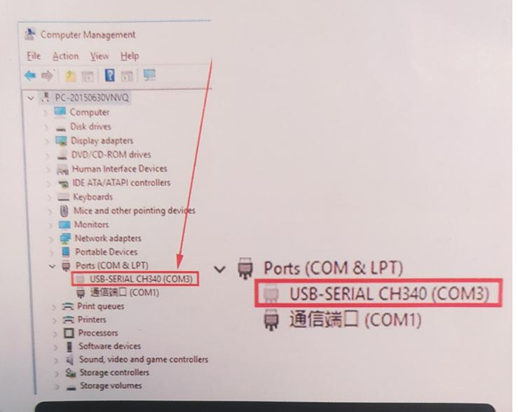
Connect the Controller to the USB port and find it on the Device Manager. It can be COM3, COM4 or COM5 .... Depends on your device
